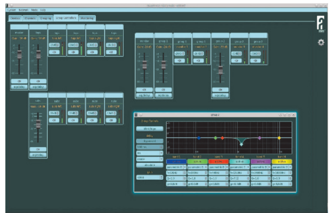
Control surface of the ALControl software with Groups and EQ windows (Fig.3)
