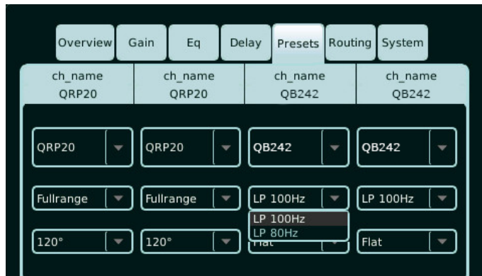
Fig 5. Range selection Select fullrange or HP at 80Hz or 100 Hz
