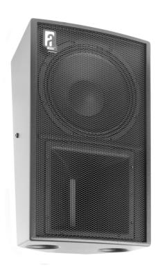
The CRS12GT/60 system consists of one RBN601 6" pro-ribbon driver for HF and a vented 12" midbass for LF reproduction. The CRS12GT/60 HF section has a 1000W peak power input, enabling a 1:15 dynamic range with lowest distortion from 1 kHz to beyond 20 kHz. The absence of a "compression threshold", caters for a linear tonal balance at any SPL, while the patented horizontal dispersion of the RBN601 guarantees a very stable sound field throughout the operating bandwidth.
