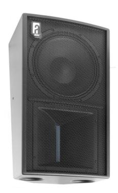
The CRS12GT/90 system consists of one RBN601 6" pro-ribbon driver for HF and a vented 12" mid-bass for LF reproduction. The CRS12GT/90 HF section has a 1000 W peak power input, enabling a 1:15 dynamic range with lowest distortion from 1 kHz to beyond 20 kHz. The absence of a "compression threshold", caters for a linear tonal balance at any SPL, while the patented horizontal dispersion of the RBN601 guarantees a very stable sound field throughout the operating bandwidth.
