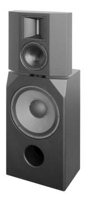
Each CRMS system consists of a separate mid-high frequency section, featuring one RBN401 4" proribbon driver HF with non-vented 8" MF and vented 15" low frequency section with low power-compression 4" voice-coil design.
